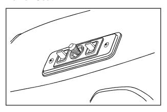
If your vehicle has front power seat(s), you can adjust them with these controls located at the front center of the seat cushion.
